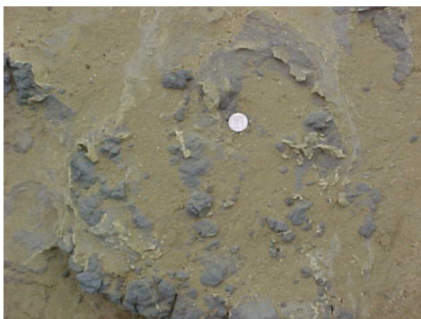
Fig. 4 The presence of jarosite mineral (yellowish color) in acid sulfate soils horizon
